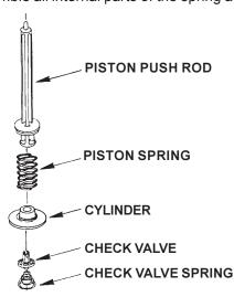
7. Insert assembly into shell. Make sure cylinder, spring and piston are nested over diffuser.
