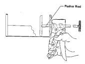
4. When the bottle is empty turn the pusher rod 180 degrees (teeth up) and pull rod all the way back. Lift out the empty bottle and replace it with a full one. See Figure 8.
