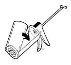
2. Turn the pusher rod 180 degrees (teeth down) to engage the teeth on the pusher rod with the mechanism in the handle and trigger assembly. See Figure 6.
